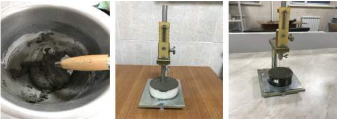
Figure 1 – Setting time test for cement paste
