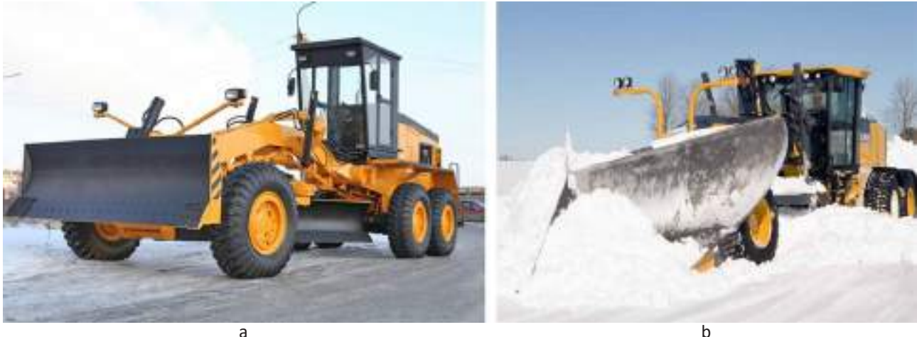
a) grader; b) grader with snow-clearing equipment
