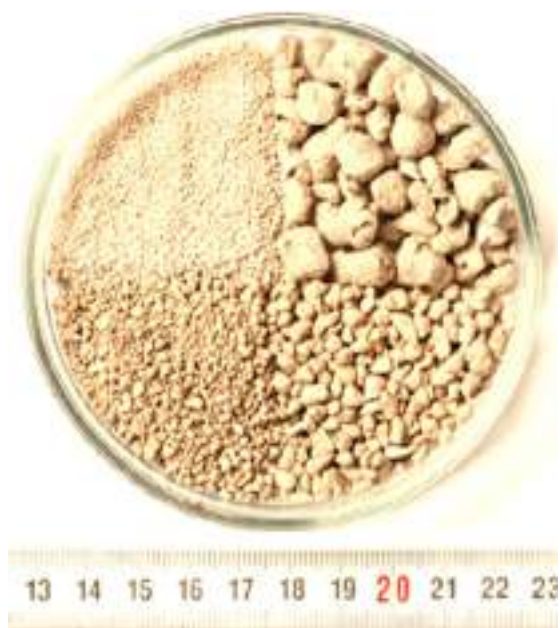
Figure 1 – Appearance of granular foam glass ceramics
